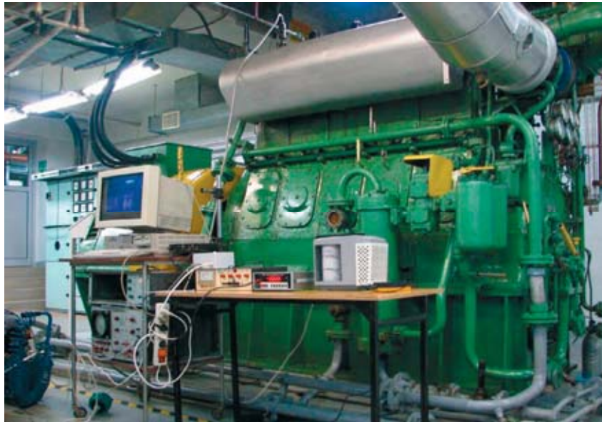
Fig. 1. The measuring stand of engine type 5BAH22
